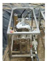
One of the more recent BrightWater projects took place at BP's Tangri field in Pakistan. The client needed surfactant deployed in order to flush and clean the rock formation; this surfactant had to run in parallel with a high viscose polymer at half the rate for the same duration. CheckPoint Pumps & Systems' solution came in the form of dual 8428 model pumps, pumping 15,850 gallons (60,000 L) into each well over a period of time at varying pressures up to 1,000 PSIG (70 BARG).
