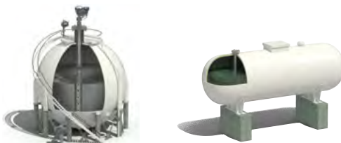
Figure 7.3: Spherical and horizontal tanks used for storing LPG.
