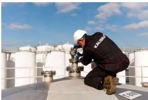
Figure 2.2: Hand gauging with a dipping tape.
