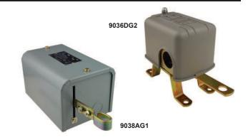
Fig. 9038-AG1 alternates two pumps and operates both pumps at once if water level rises above normal high level. It requires magnetic starters unless the pump motors are single phase. 1 HP, or smaller and have overload protection.
