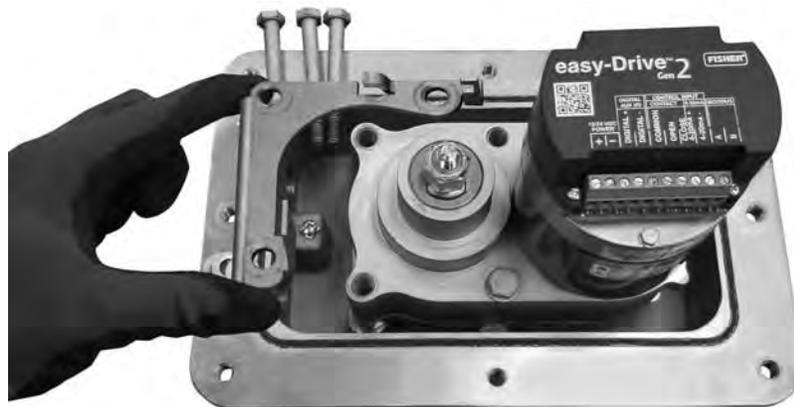
3. Use the motor housing bolts removed in step one to secure the mounting bracket in place. Note the washers will not be used with the bolts with the mounting bracket.
