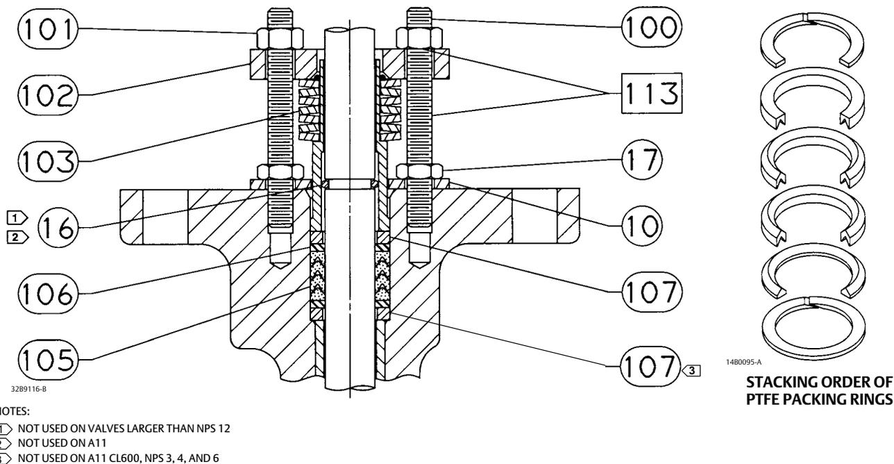
11. Install the packing flange (key 102) on the shaft, and install the packing nuts (key 101). Hand tighten them.
